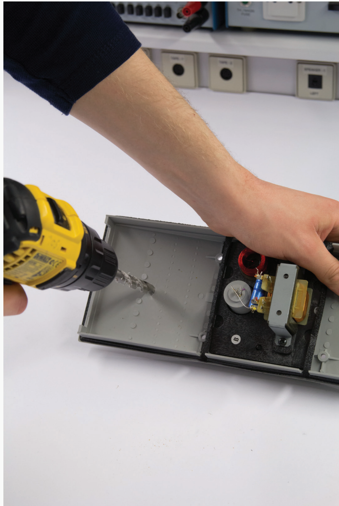
Drill a 11 mm hole in the desired location of the back plate.
