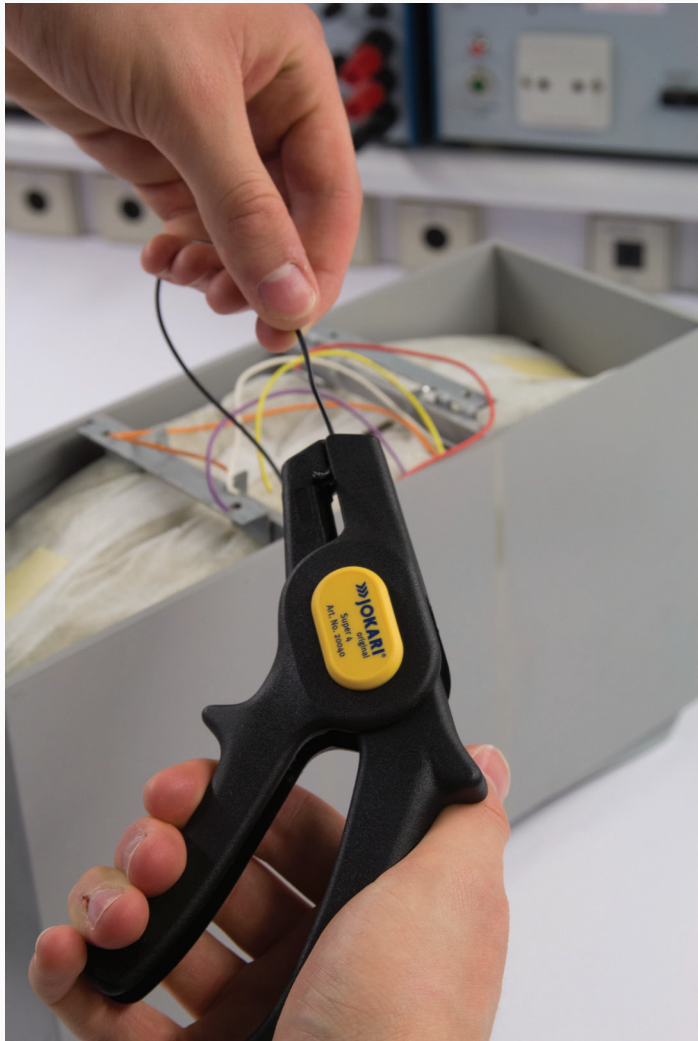
Strip the ends of the speaker wires, so that approximately 1cm of wire is exposed.
