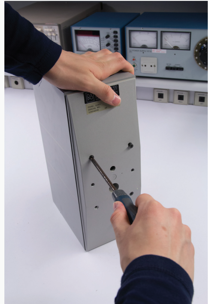
Screw on the back plater with the four screws.
