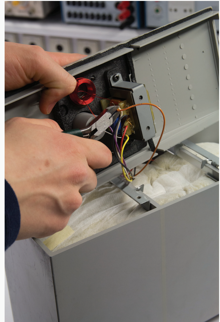
Cut the wires connected to the back plate.
