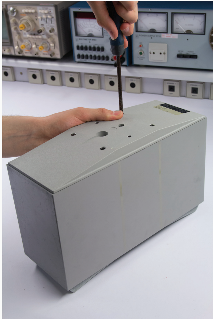
Unscrew the back plate of the factory CX100.
