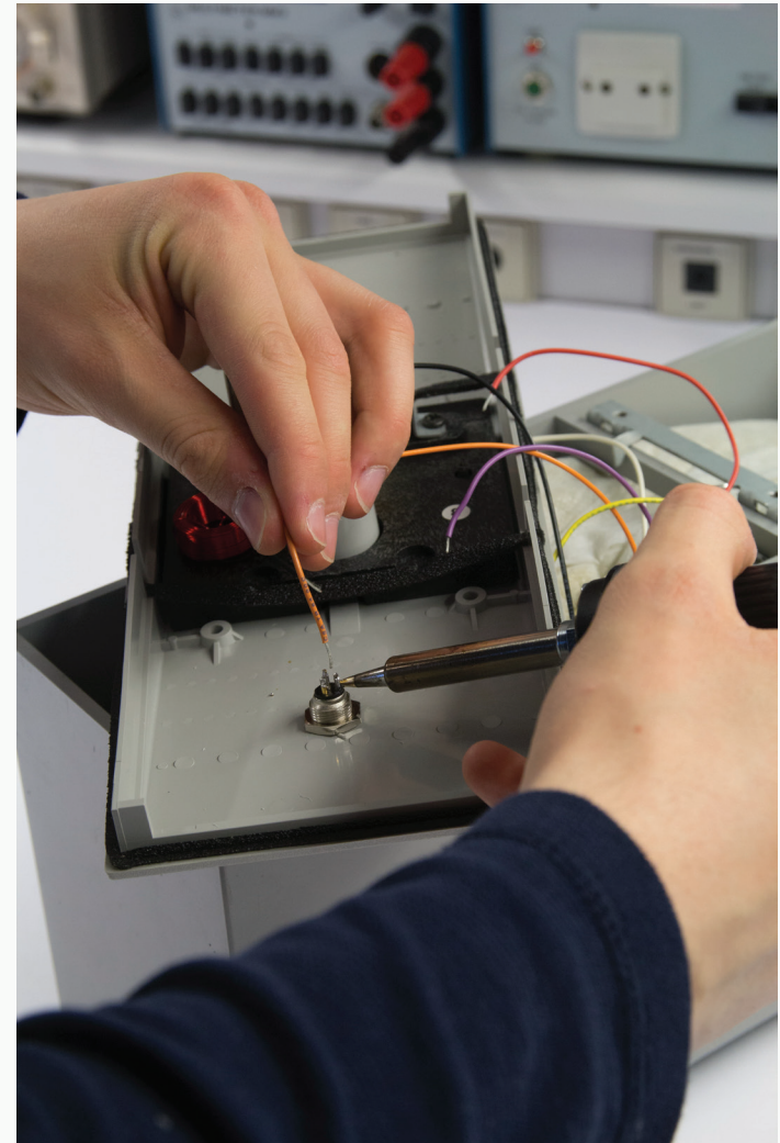
Solder the four wires to the XLR plug installed earlier. A detailed diagram is located on the next page.
