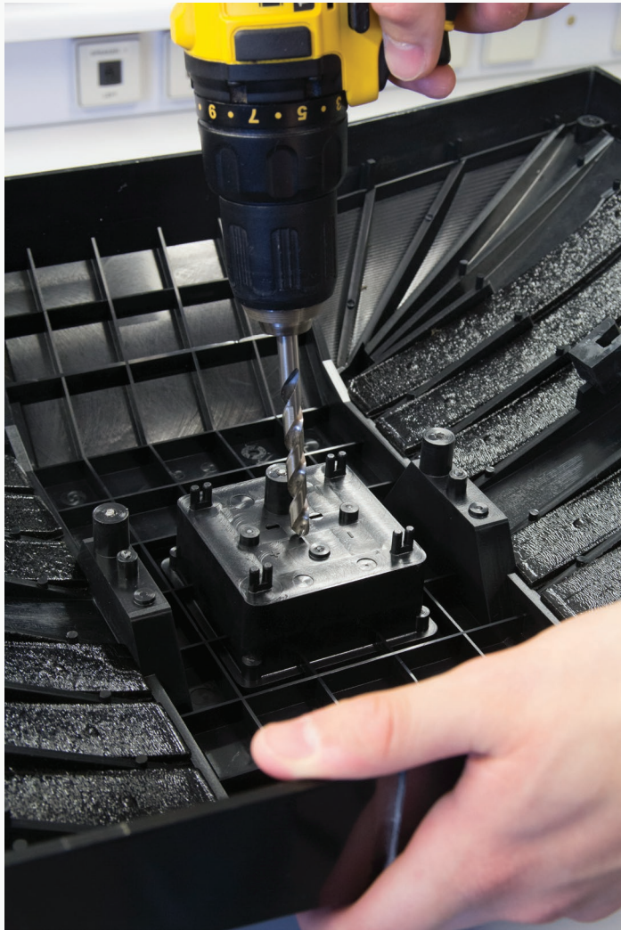
Drill a 8mm hole where the previous connections were located.
