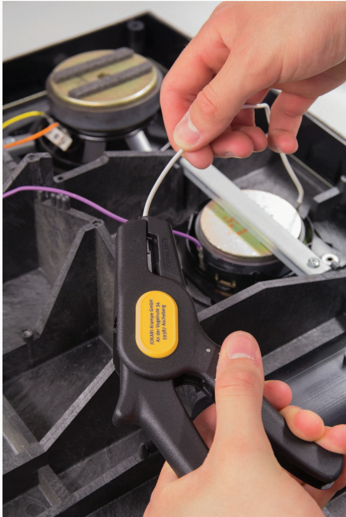
Strip the wires coming from the drivers, so that again approximately 1 cm of wire is exposed.
