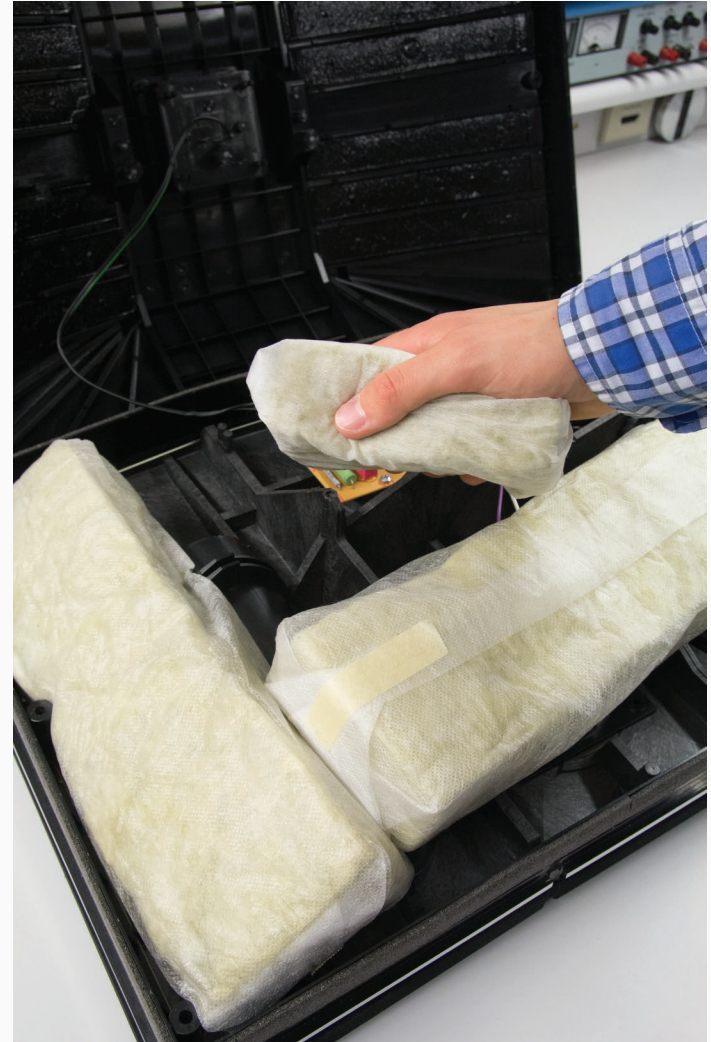
Open up the back plate and remove the dampening material.
