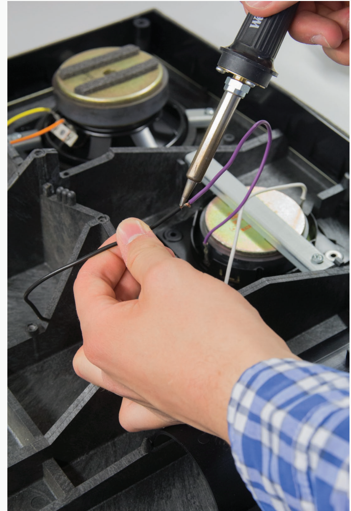
The tweeter will require an extension to be soldered onto it.
