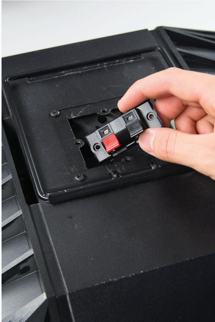
Whilst being on the back of the speaker, unscrew the old connectors.
