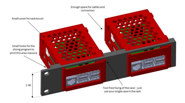
The rackmount is designed to print it in a printer like the Anycubic i3 mega with a printing area of 210 mm x 210 mm. Of course, you can also use the rackmount with only one raspberry pi.
