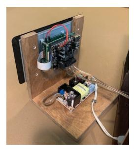
I had a RPi 3B, laying around. I bought the excellent Hifiberry Amp 2 (~\$50), an official Raspberry Pi 7 inch Touchscreen (<\$70), and a 60W (Meanwell RPS-60-15, \$16) power supply. It all stacked up into a pretty small package.
